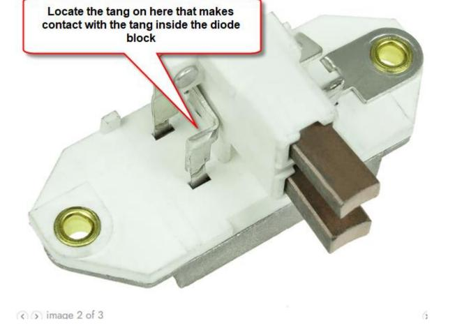
Once that is located correctly, then solder a 120mm Blue wire and route outside the alternator. This is now P switching FIELD control.
