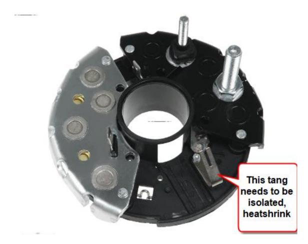
Failure to isolate this will negate the external regulator controlling the positive brush, you can also bend down the tang but it can sometimes break off. I normally apply two lots of heat shrink tube
