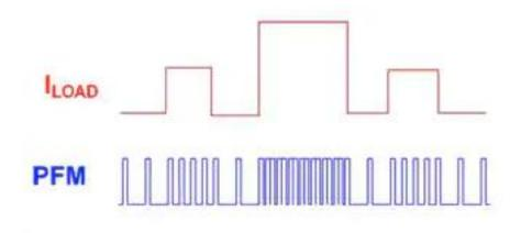
Graph showing pulse frequency modulation versus load.
