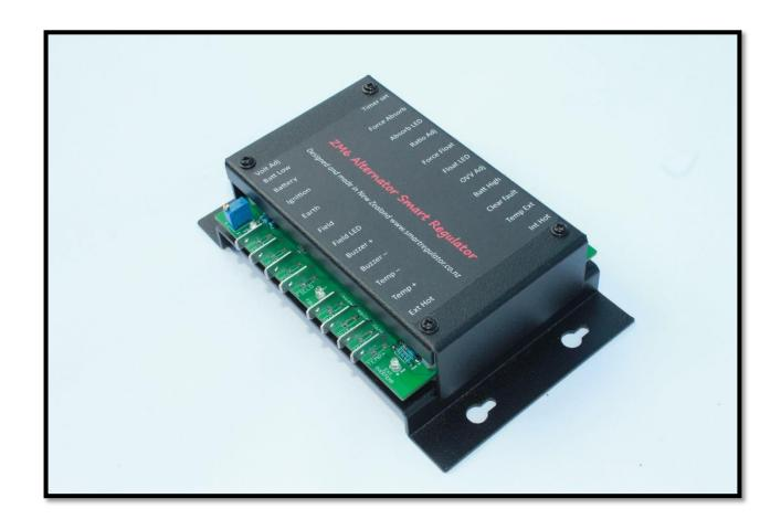
Alternator (Adjustable) Voltage Regulator – ZM6
